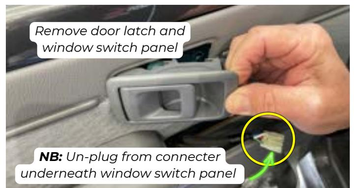
Remove the Phillips head screw securing the door latch, then carefully proceed to remove the Door Latch and the Power Window Switch Panel using a plastic trim removal tool.
