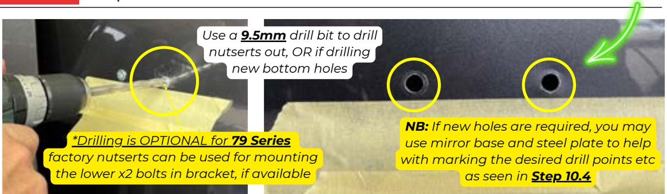
**9.1** If drilling is required, locate the 2 bottom holes on the exterior of vehicle.
