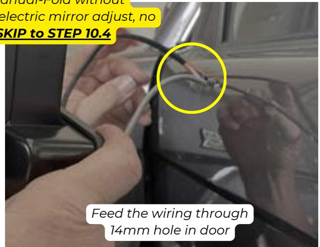
**10.1** Remove the Plastic Lining from the interior slightly, and let it hang, then feed the wiring through the rubber grommet supplied in the kit.
