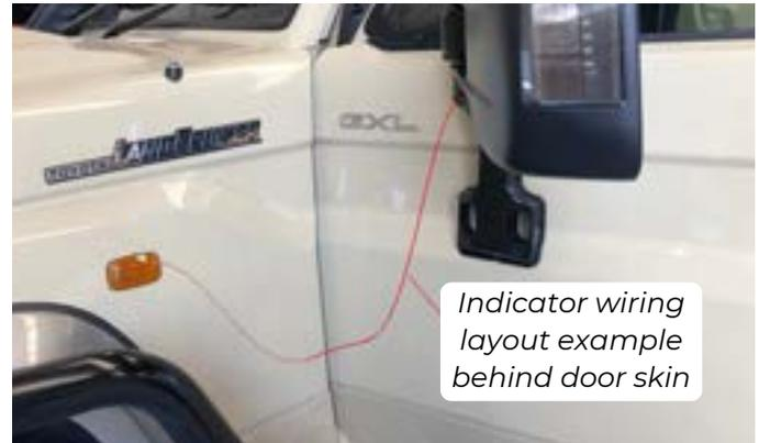
**13.1** Remove the 70 Series side factory indicator out, then locate the **positive** and **negative** wires.
