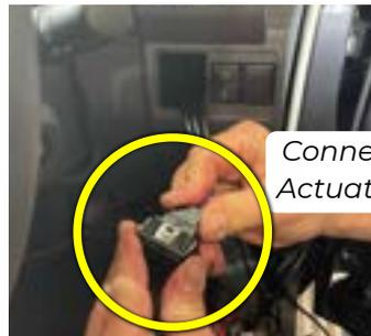
Connect Mirror Actuator wiring
