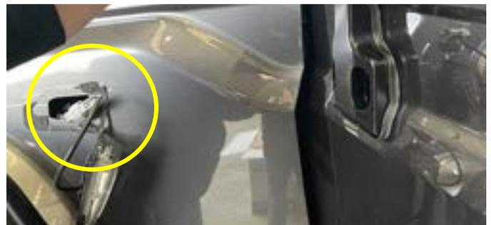
**13.2** When tapping into the side indicator wires in the vehicle guard (bare wire end of kit):
