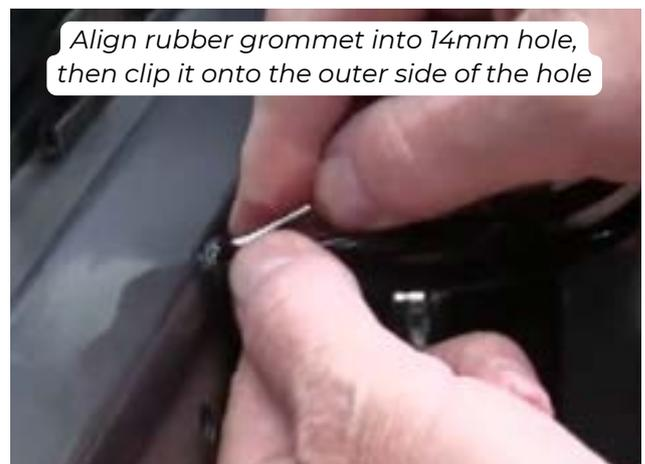
**10.3** Once you have met the rubber grommet, align the rubber grommet into the 14mm hole, then clip it onto the outer side of the hole.
