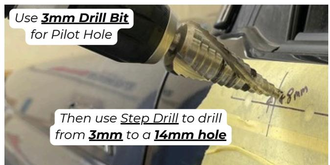
**8.2** Once you have drilled the 14mm hole, you can then discard the masking tape.
