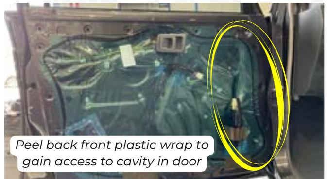
Pry back the door trim using a plastic trim removal tool. Start from the bottom corner, then work your way along the panel to pry back the rest of the door trim.
