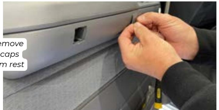
Take extra care by gently removing the Square caps from the door handles. Use a plastic trim remover tool (or a very thin flat screwdriver) to pry the piece back, then use a Phillips screwdriver to remove the screws securing the trim to the door.
