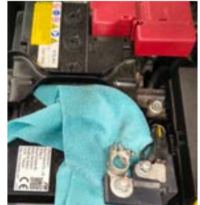
Cover the battery connectors with a fabric cloth to prevent accidental contact with the negative (-) battery terminal.
